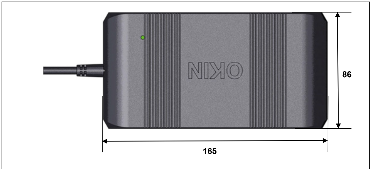
Figure 3 Dimensions of the CU165, top view (in mm)
