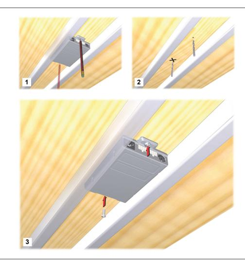
Figure 33 Mounting the SMARTeco control unit
