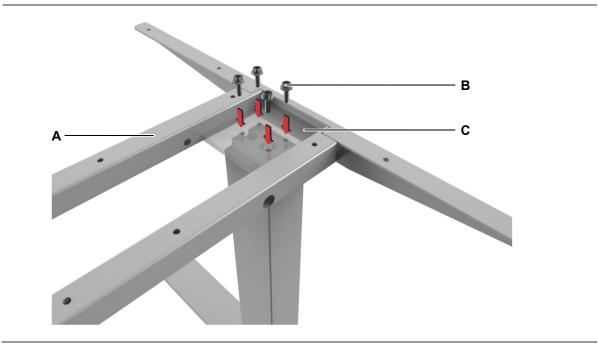
Figure 20 Mounting the table frame
