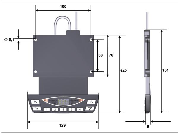
Figure 26 HSF control keypad, installation dimensions (in mm)
