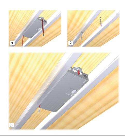
Figure 37 Mounting the COMPACT control unit
