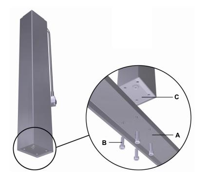
Figure 18 Mounting the table base:
