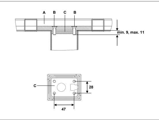
Figure 19 Mounting the table frame (dimensions in mm)
