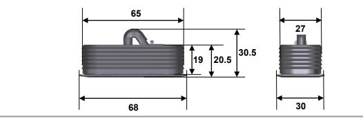
Figure 27 TOUCHbasic-inlay keypad, mounting dimensions (in mm)
