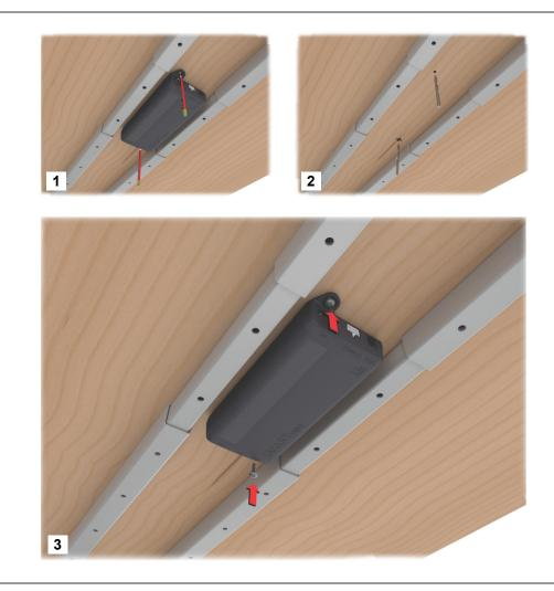
Figure 35 Mounting the SMARTneo / SMARTneo-pro control unit
