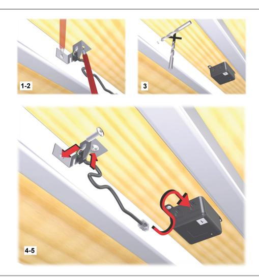
Figure 44 Mounting the sensor unit (sensor and processor)
