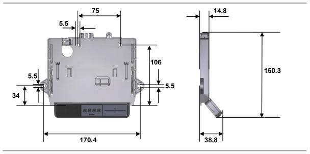
Figure 30 TOUCHdown keypad, mounting dimensions (in mm)
