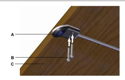
Figure 22 Example: Mounting the Motion Assist control keypad
