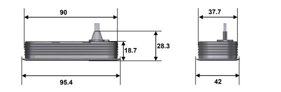
Figure 31 TOUCHinlay keypad, mounting dimensions (in mm)
