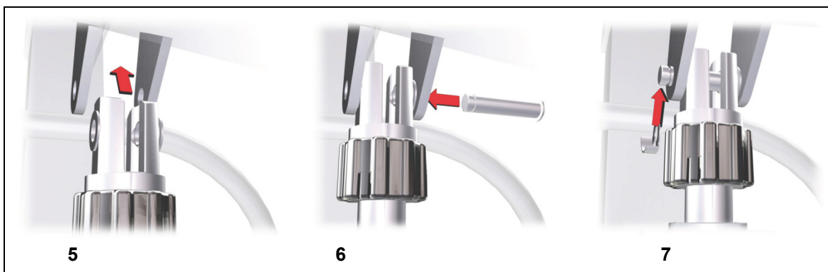
Figure 24 Steps for installing the LR clevis (example)
