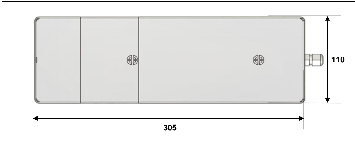
Figure 4 Dimensions of the AG300, top view (in mm)
