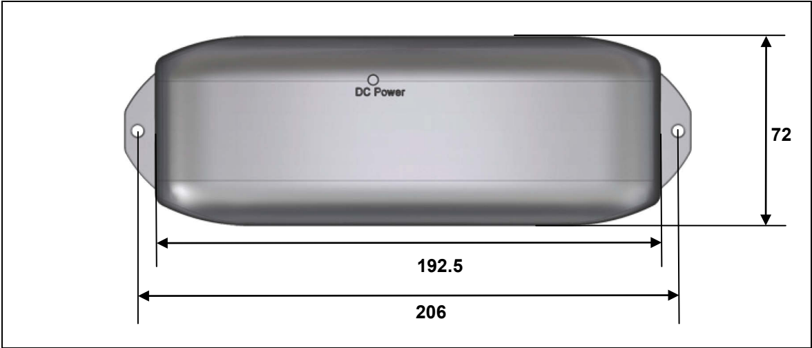
Figure 5 Dimensions of the PD18 POWER SUPPLY, top view (in mm)
