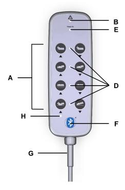
Keypad of the IPROXX 2 handset, with 8 movement keys and Bluetooth®
