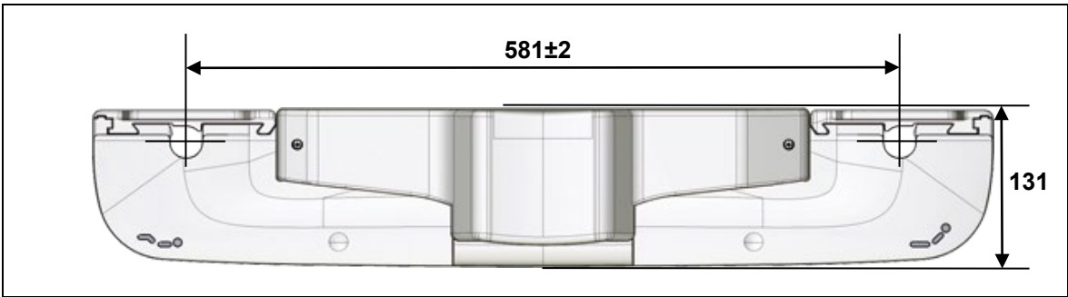
Figure 10 Dimensions of the DUOMAT 9 drive, in mm
