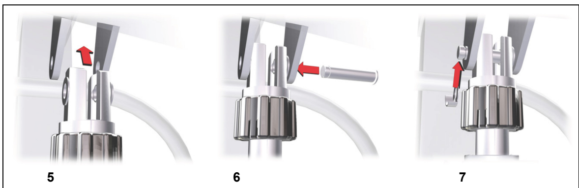
Figure 24 Steps for installing the LR clevis (example)
