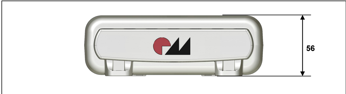
Figure 7 Dimensions of the MCL III control unit, front view (in mm)
