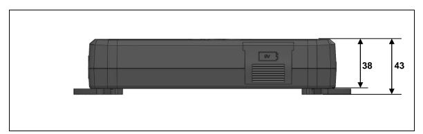
Figure 9 PD21, side view (in mm)
