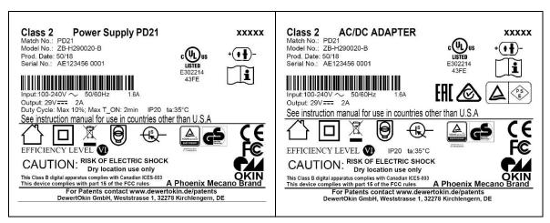
Figure 2 Example: Ratings plate for the PD21
