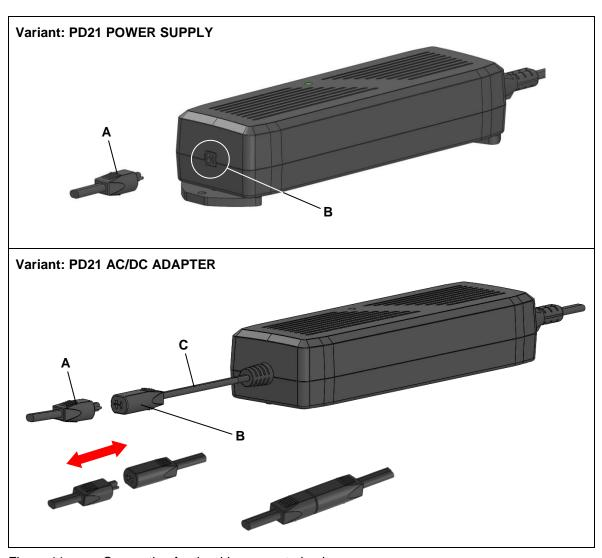
Figure 11 Connection for the drive or control unit
