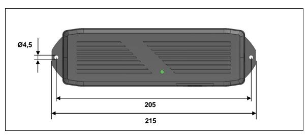
Figure 8 PD21 POWER SUPPLY, top view (in mm)
