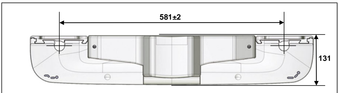
Figure 10 Dimensions of the DUOMAT 9 drive, in mm
