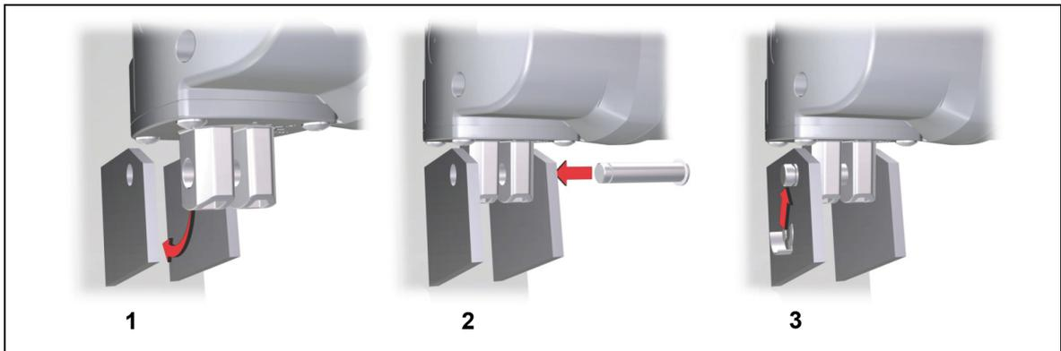
Figure 23 Steps for installing the gear clevis (example)
