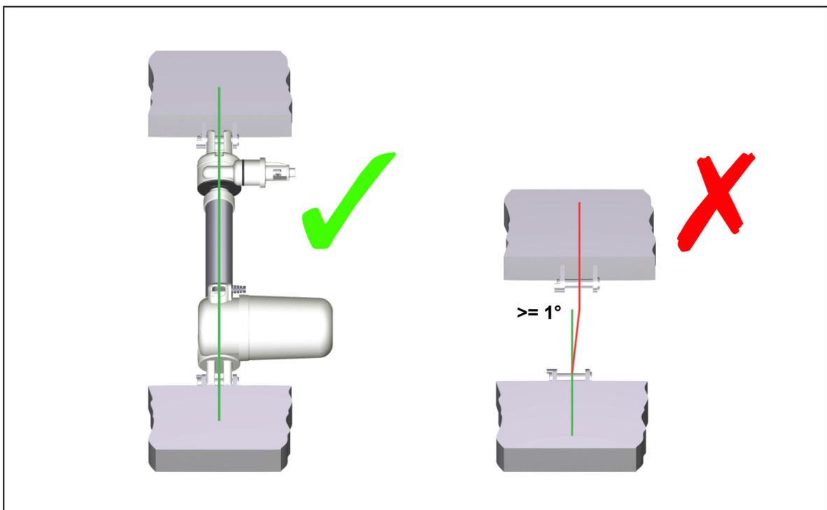
Figure 17 Position and alignment of the brackets
