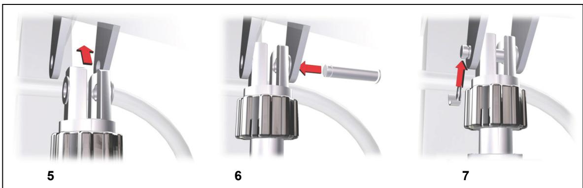
Figure 24 Steps for installing the LR clevis (example)
