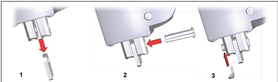
Figure 15 Steps for installing the gear clevis (example)
