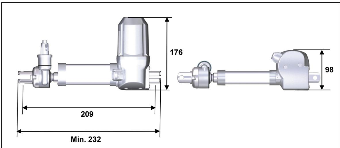
Figure 12 Dimensions of MEGAMAT MFZ drive with GQR (in mm), minimum installation dimensions: 209 mm
