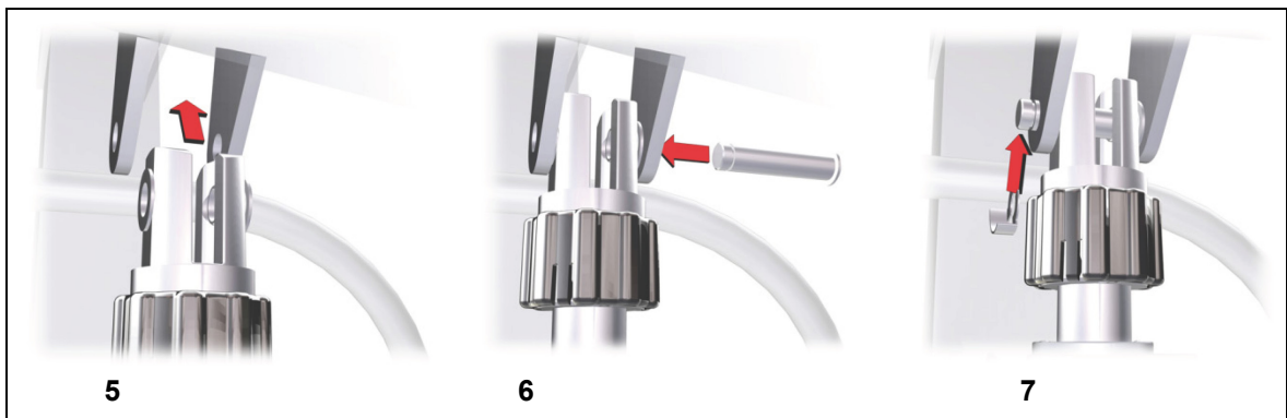
Figure 24 Steps for installing the LR clevis (example)
