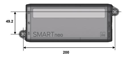
Figure 41 Mounting dimensions: SMARTneo / SMARTneo-pro control unit (in mm)
