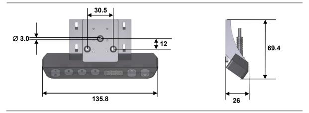
Figure 32 HSU control keypad, installation dimensions (in mm)
