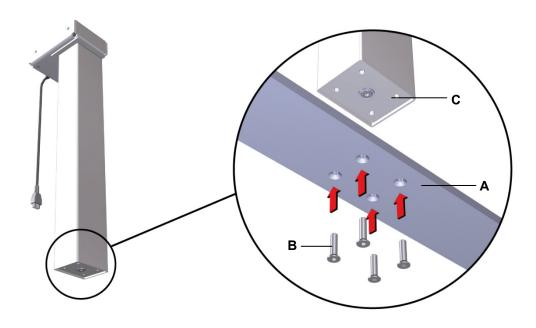
Figure 25 Example: Mounting the table base (for variant D)
