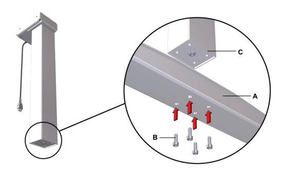
Figure 21 Example: Mounting the table base
