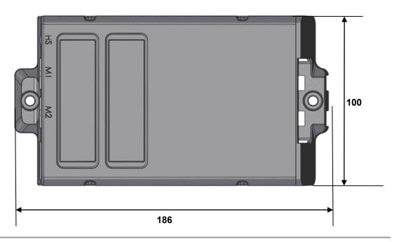
Figure 64 SMARTeco control unit, top view (in mm)
