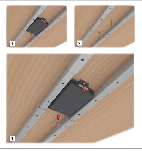
Figure 40 Mounting the SMARTeco control unit
