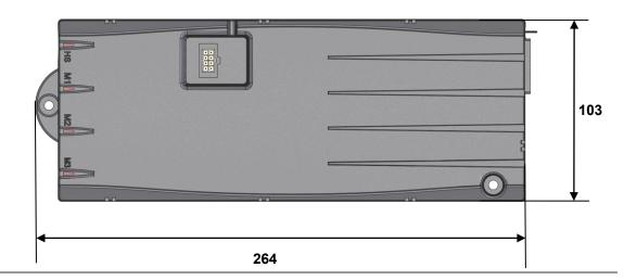
Figure 68 SMART control unit, top view (in mm)
