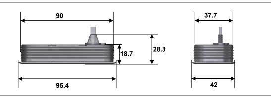
Figure 38 TOUCHinlay keypad, mounting dimensions (in mm)
