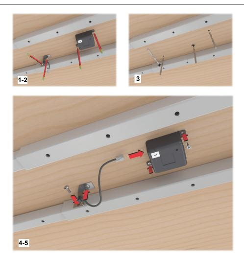
Figure 51 Mounting the sensor unit (sensor and processor)
