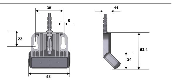
Figure 35 TOUCHbasic-down keypad, mounting dimensions (in mm)
