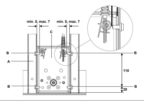
Figure 26 Example: Mounting the table frame (dimensions in mm)
