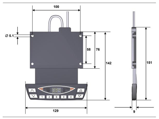
Figure 33 HSF control keypad, installation dimensions (in mm)
