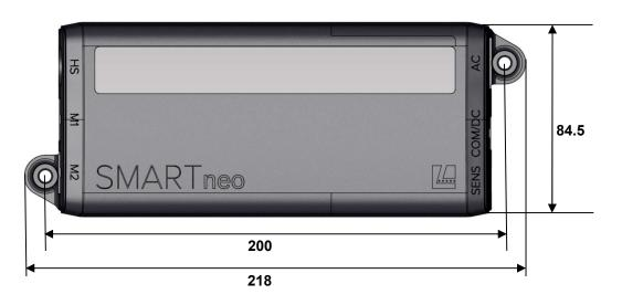
Figure 66 SMARTneo / SMARTneo-pro control unit, top view (in mm)
