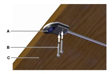
Figure 29 Example: Mounting the Motion Assist control keypad
