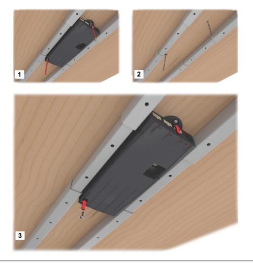
Figure 44 Mounting the COMPACT control unit
