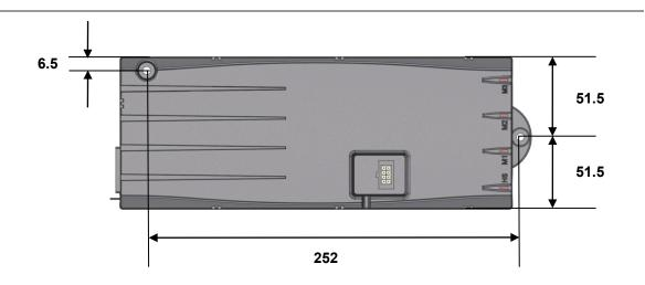
Figure 43 Mounting dimensions: COMPACT control unit (in mm)
