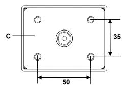
Figure 22 Mounting the table base (version B) (in mm)
