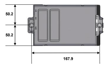
Figure 39 Mounting dimensions: SMART control unit (in mm)
