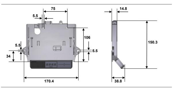
Figure 37 TOUCHdown keypad, mounting dimensions (in mm)
