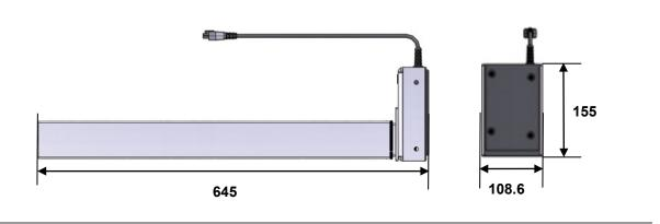
Figure 70 DD11S lifting column (in mm)
