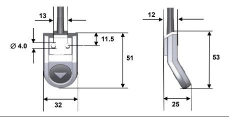
Figure 28 Motion Assist control keypad, installation dimensions (in mm)
