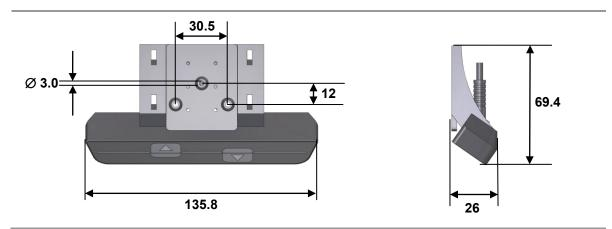
Figure 31 HSU Varioline control keypad, installation dimensions (in mm)
