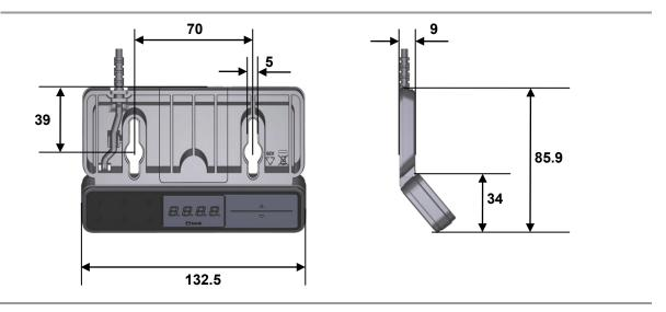
Figure 36 TOUCHfx keypad, mounting dimensions (in mm)
