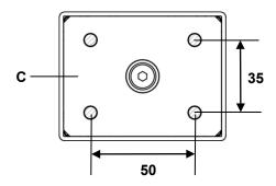
Figure 24 Mounting the table base (version D) (in mm)
