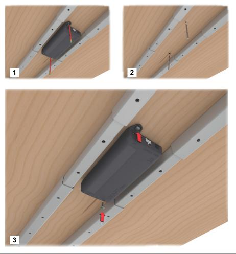
Figure 42 Mounting the SMARTneo-pro control unit
