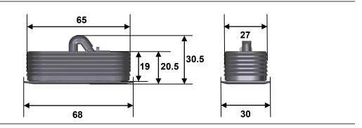
Figure 34 TOUCHbasic-inlay keypad, mounting dimensions (in mm)
