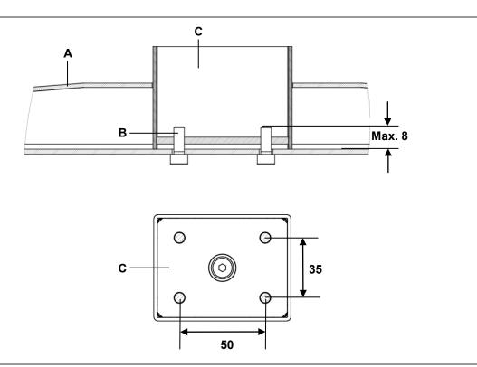
Figure 20 Mounting the table base (version A) (in mm)
