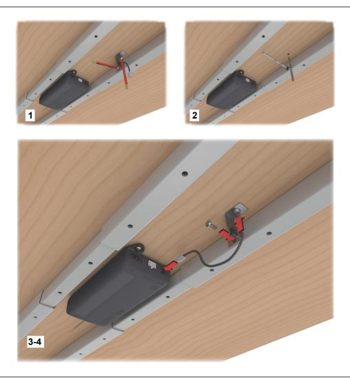
Figure 49 Mounting and connecting the sensor to the SMARTneo-pro control unit
