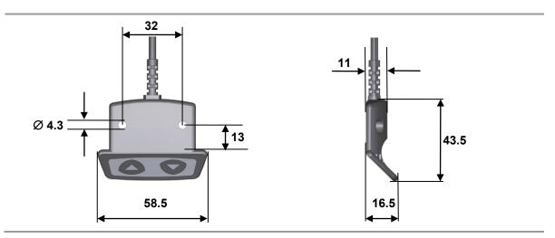
Figure 30 HSCO control keypad, installation dimensions (in mm)
