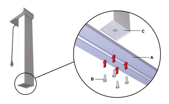
Figure 23 Example: Mounting the table base (version B)
