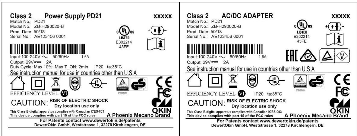
Figure 2 Example: Ratings plate for the PD21
