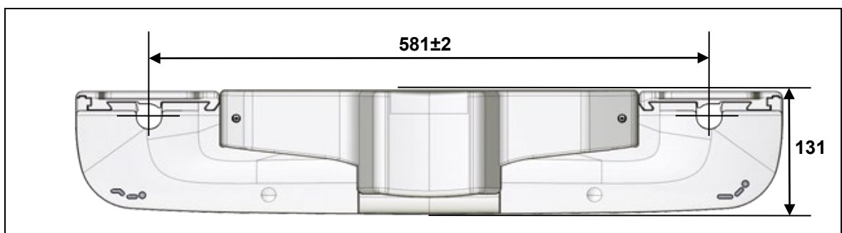
Figure 10 Dimensions of the DUOMAT 9 drive, in mm
