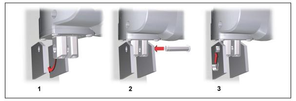
Figure 23 Steps for installing the gear clevis (example)
