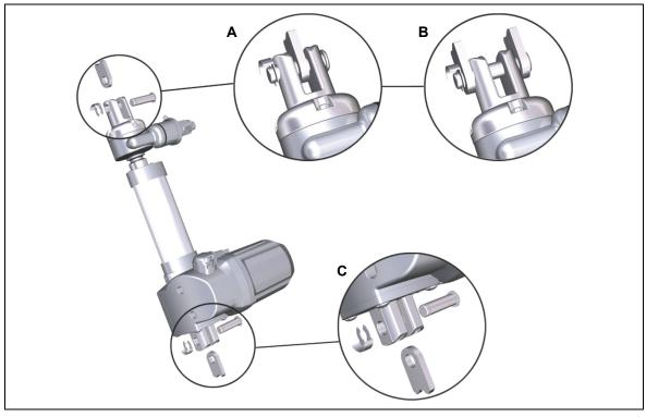
Figure 19 Recommended design of bracket
