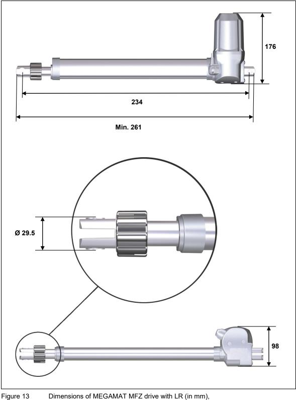
Dimensions of MEGAMAT MFZ drive with LR (in mm), minimum installation dimension: 234 mm
