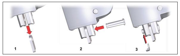
Figure 15 Steps for installing the gear clevis (example)
