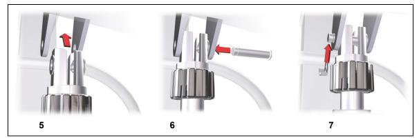
Figure 24 Steps for installing the LR clevis (example)
