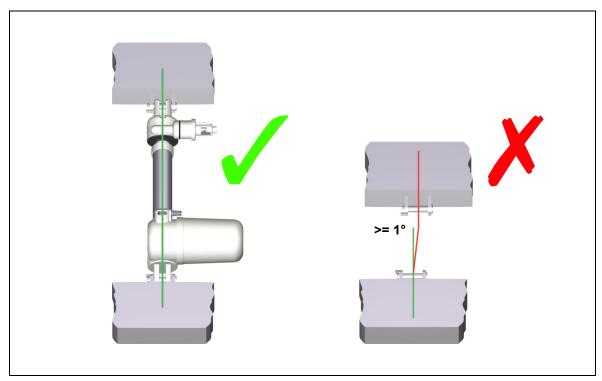
Figure 17 Position and alignment of the brackets
